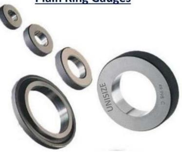
Plain Ring Gauges used for the attribute inspection of outer diameter of shafts, pipes, etc. whereas the master setting ring gauges are used to set the inspection instruments like bore gauge, universal length measuring machine, etc. We supply the plain ring gauges and master setting ring gauges in the below options,
