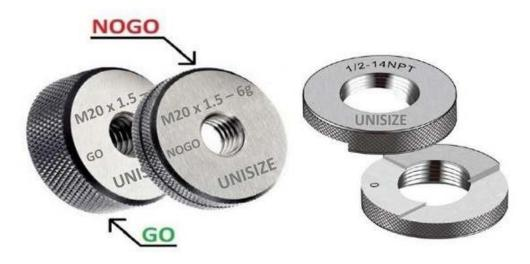
"Thread Ring Gauges" are the type of fixed limit gauges used for attribute Inspection of outer diameter of threaded shafts, pipes, or any cylindrical component with external threads. We supply the thread gauges of the below types. Information regarding size, pitch, etc. will be provided upon request.
